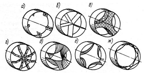
Figure 7: Designs of inner heat exchangers of rotary kilns
