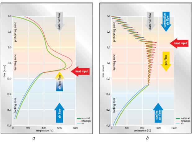
*a* – common shaft kiln; *b* – PFR kiln Maerz
