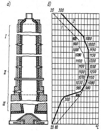
a) zones of shaft kiln: I – preheating, II – calcining and III – cooling
