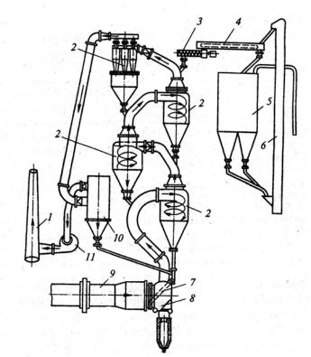
Figure 9: Scheme of external cyclone heat-exchanger
