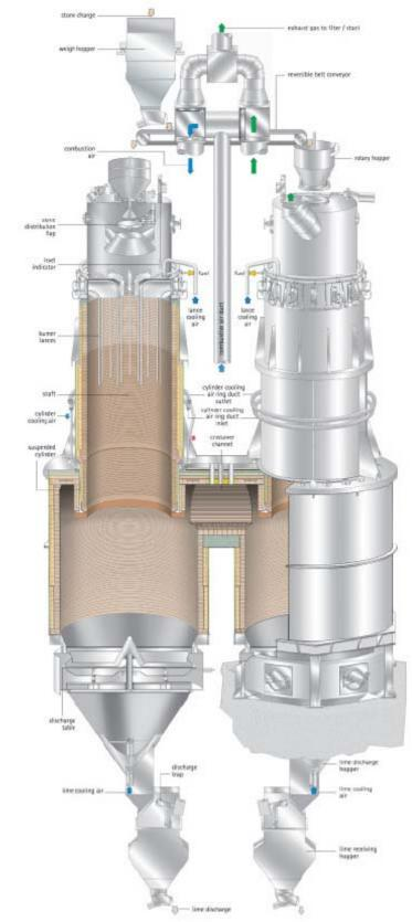
Figure 5: Appearance of kiln PFR for calcining fine limestone
